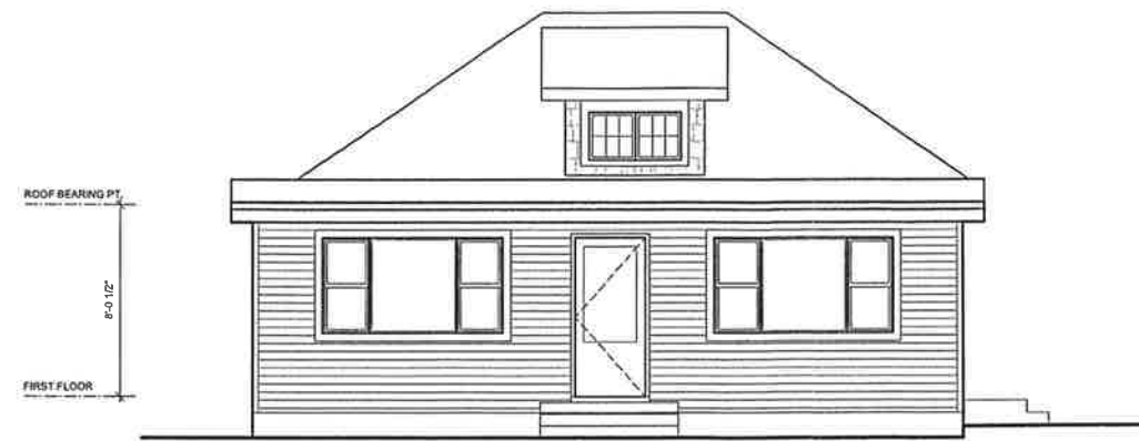
2 EXISTING SIDE (EAST) ELEVATION SCALE: 1/4" = 1'-0"
